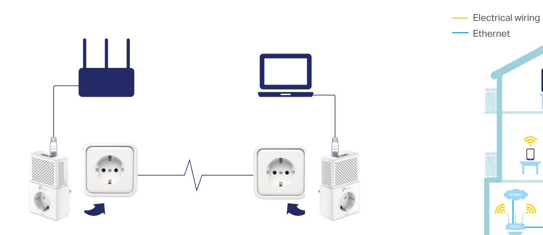
Powerline adapters and extenders must be deployed in a set of two or more.
